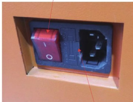
Use a flat-head screwdriver to gently pry up the side latch — the fuse is located inside.
