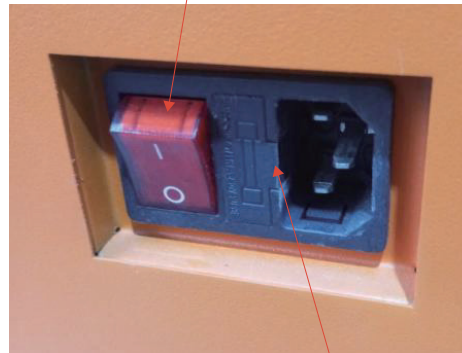
Power switch: With built-in indicator light
